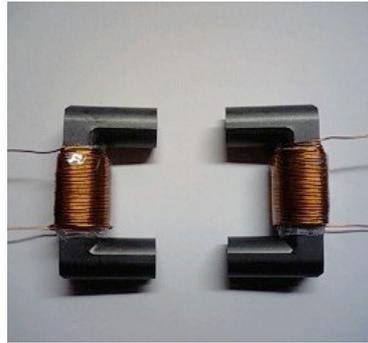
Fig.1 Tested transformer employing U shape ferrite cores.
