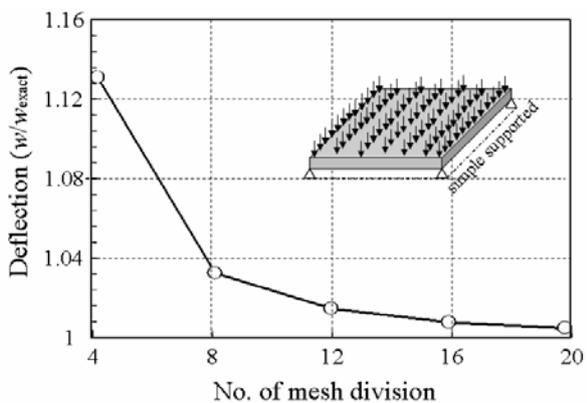
Fig.14 Ratio of deflections by exact and HPM when Poisson Ratio=0.2
