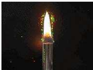
Yellow shows 1/f fluctuation points Fig.4 1/f fluctuation accompanying gas burning
