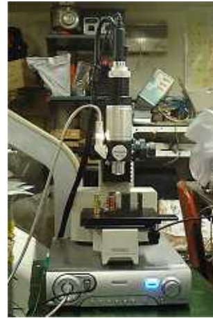
Fig.9 Experimental device for magnetic wall observation.
