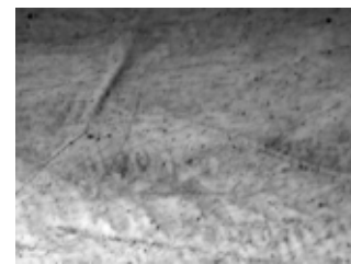
Fig.3 Static Magnetic Domain Image derived as an average of entire frame images in Fig. 2
