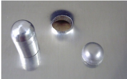
Fig.9 Back view of target. (target thickness=3mm)
