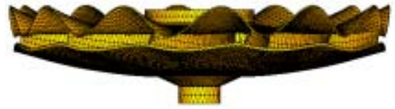
Fig.7 Deformation by centrifugal force
