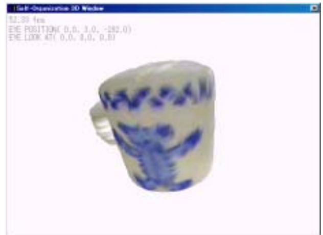
Fig.4 3D graphics constructed from 3 photographs of Fig.3.
