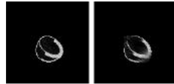
Fig. 2. Reconstructed images vs. data acquisition area. (left: Fig.1(a) 360 \text{ deg.} , right: Fig.1(c) 90 \text{ deg.} )
