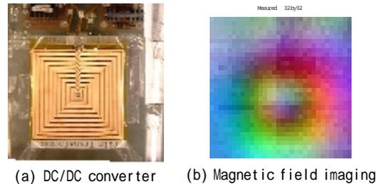
Fig. 5 DC/DC converter using film-type transformer
